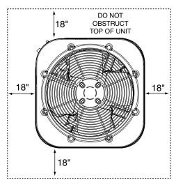
Figure 1. Clearance Requirements
