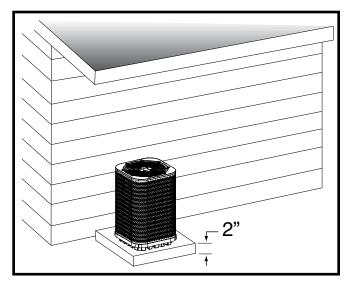
Figure 2. Ground Level Installation
