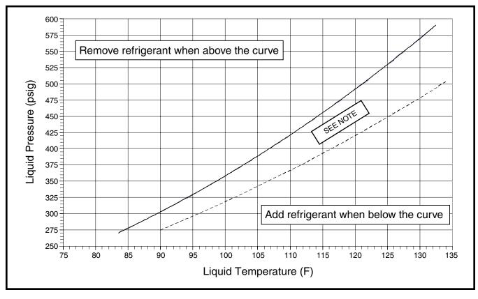
Figure 7. Charging Chart for S4BD-036 Series (3 Ton Units) - TXV Matches
