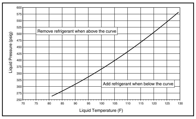
Figure 10. Charging Chart for S4BD-060 Series (5 Ton Units) - TXV Matches
