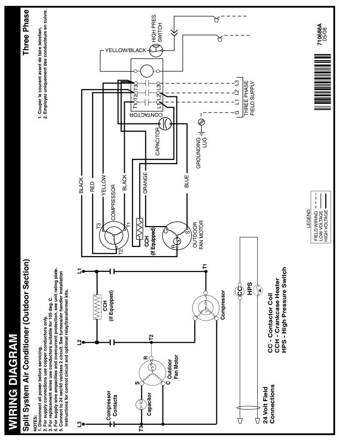
Figure 12. Wiring Diagram for S4BD, 3- Phase Models (3, 4, & 5 Ton Units)
