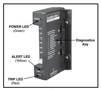
Figure 3. Comfort Alert™ Diagnostics Module
