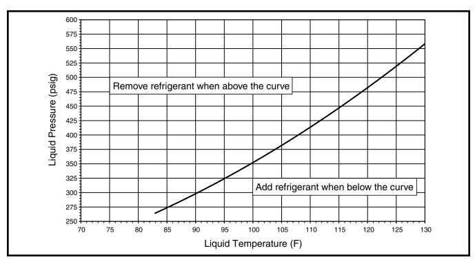
Figure 4. Charging Chart for S4BD-018 Series (1.5 Ton Units) - TXV Matches
