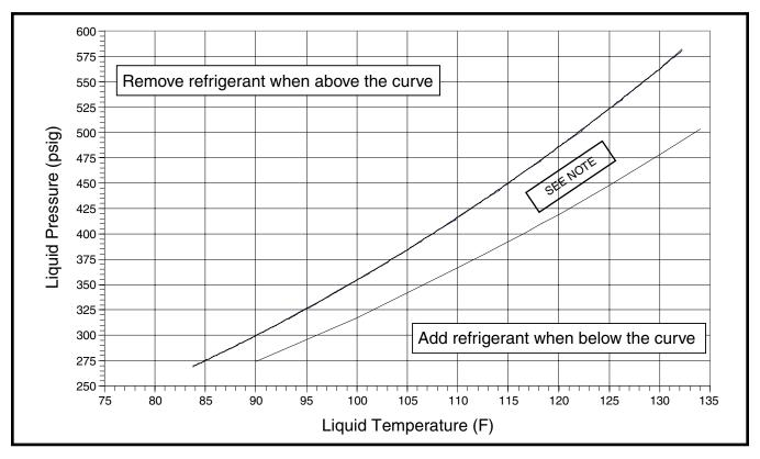
Figure 6. Charging Chart for S4BD-030 Series (2.5 Ton Units) - TXV Matches
