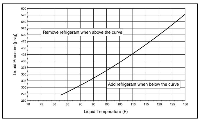
Figure 9. Charging Chart for S4BD-048 Series (4 Ton Units) - TXV Matches
