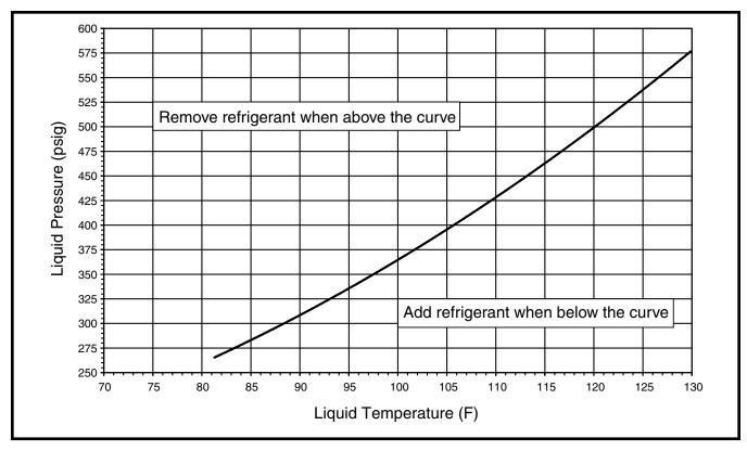
Figure 8. Charging Chart for S4BD-042 Series (3.5 Ton Units) - TXV Matches
