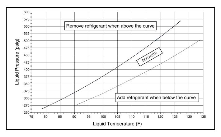
Figure 5. Charging Chart for S4BD-024 Series (2 Ton Units) - TXV Matches
